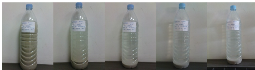
Figure 11. A simple way of measuring percentage of fines.
