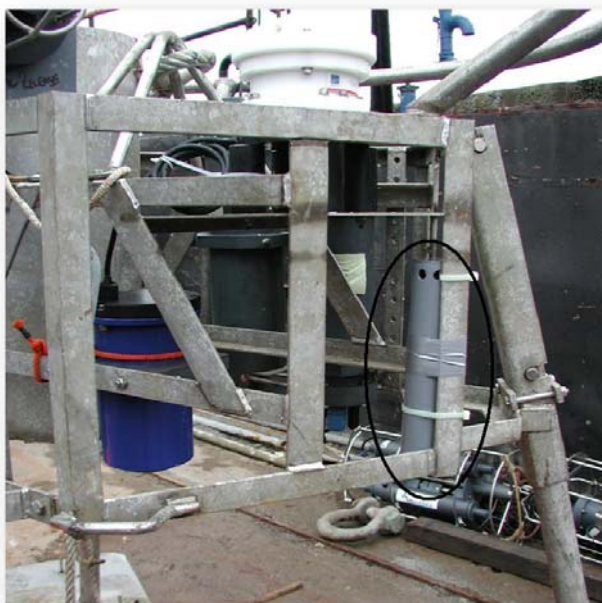
Figure 13. A Booner sediment trap (circled) mounted on a Cefas Seabed lander (MiniLander) and the design of a sediment trap.
